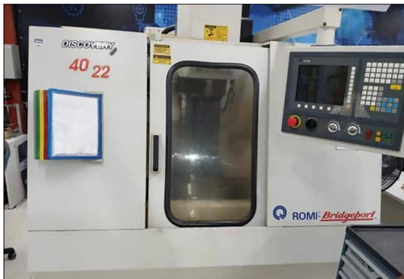
Figure 1. ROMI Discovery 4022 vertical machining center.
