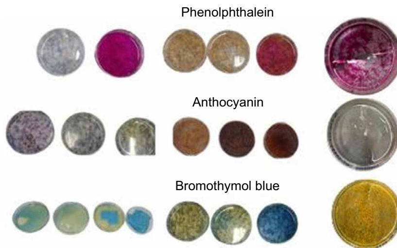
Figure 6. Formulations 1 and 3 (CMC) were contaminated with unknown microorganisms with phenolphthalein and bromothymol blue indicators, respectively.
