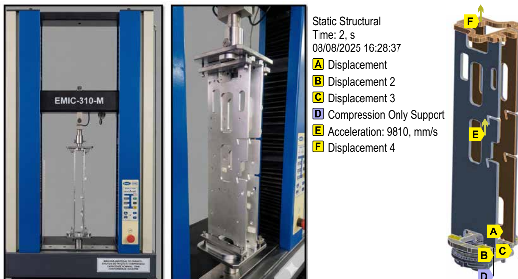
Figure 1. Experimental tensile test setup and finite element model.
