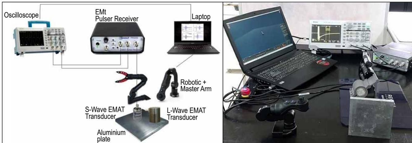
and an L-wave 5 MHz center frequency LW155T. To accommodate each EMAT transducer, a custom gripper was designed with dimensions tailored to the specific requirements of the L-wave and S-wave transducers. The movement of the gripper was controlled using the master arm of the Alpha 5 manipulator.
