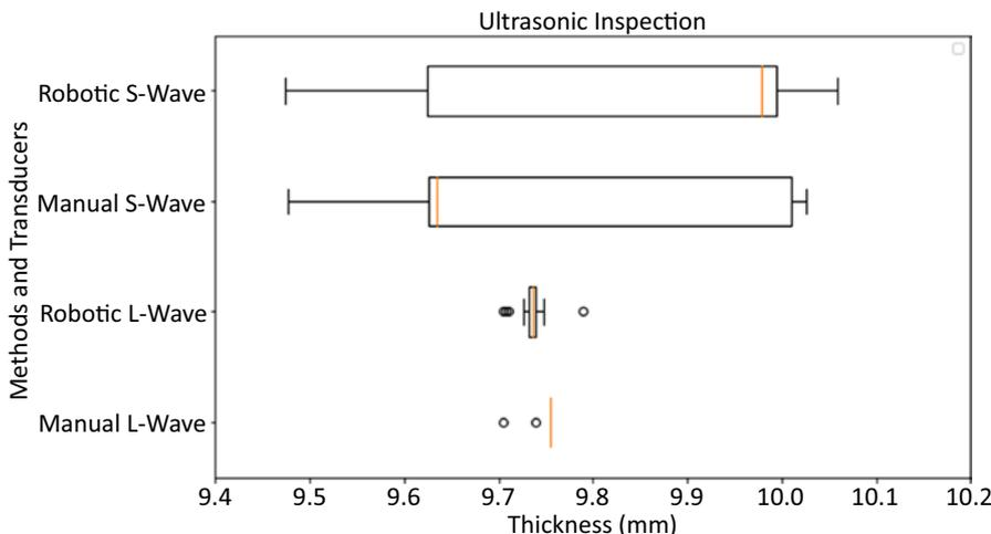
measurement accuracy for aluminum thickness. The boxplot analysis confirms that the average values obtained from the robotic signals fulfill this purpose. The robotic arm demonstrates excellent efficiency and successfully meets the high-speed inspection requirements to capture and measure the thickness of aluminum with the desired precision.
