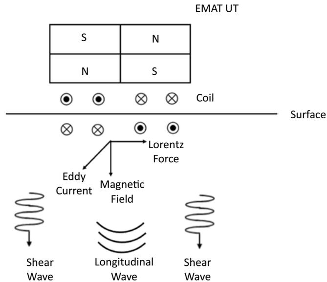
of the field [6,7]. Magnetostriction, the property of ferromagnetic materials to deform in the presence of an external magnetic field, contributes to higher energy conversion efficiency in EMATs based on magnetostriction compared to those based on the Lorentz force [10,11].
