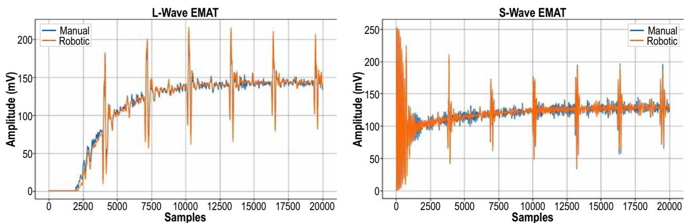
and precise application to the EMAT transducer, producing more robust and pronounced ultrasound signals. These higher signal amplitudes facilitate easier detection and analysis of reflection peaks, enabling more precise thickness measurements. Furthermore, robotic arm inspection with the Alpha 5 diminishes the likelihood of signal distortion or noise interference, leading to more reliable inspection results.
